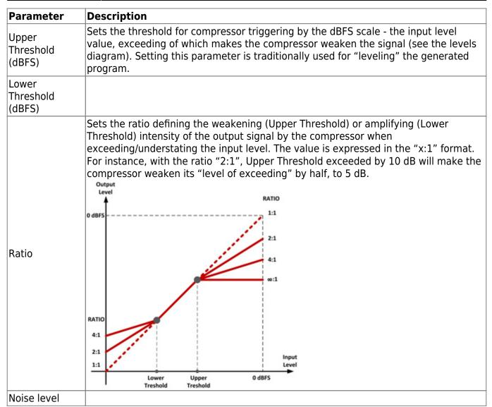
The compressor doesn't allow to adjust the **Attack time** and **Release time** parameters.
